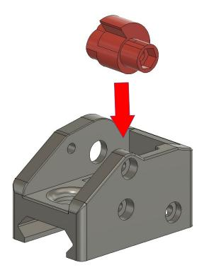
Insert Gear through Main Body into Cam.
