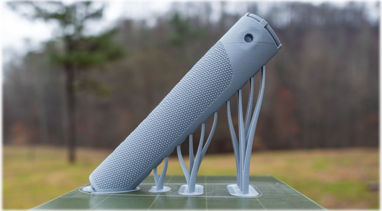
Figure 3 Handguard printed in proper orientation.
