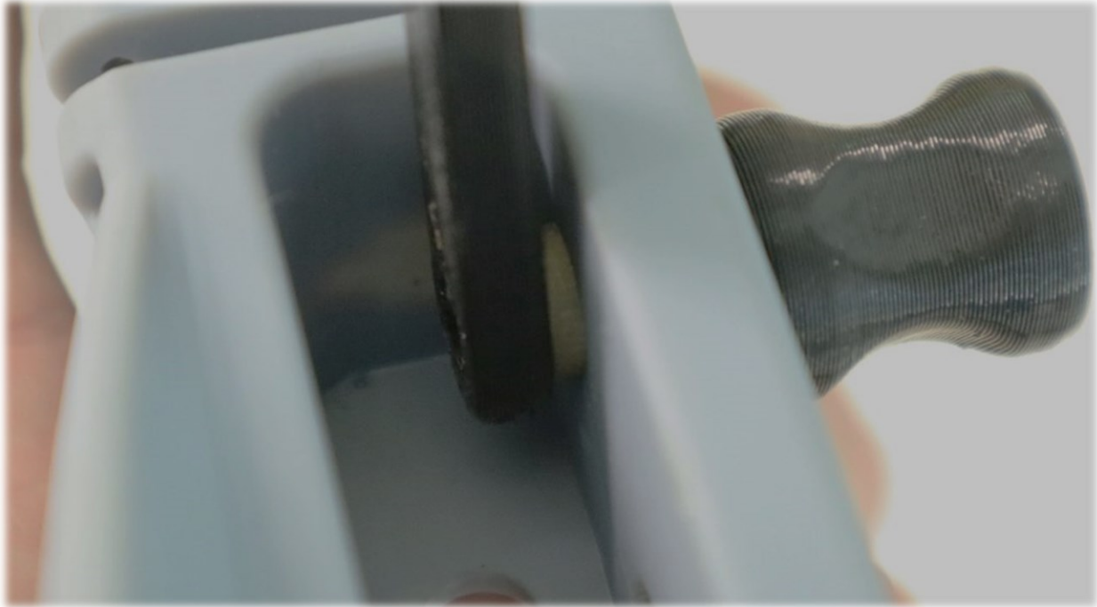
Figure 8 Installing the bushings.
