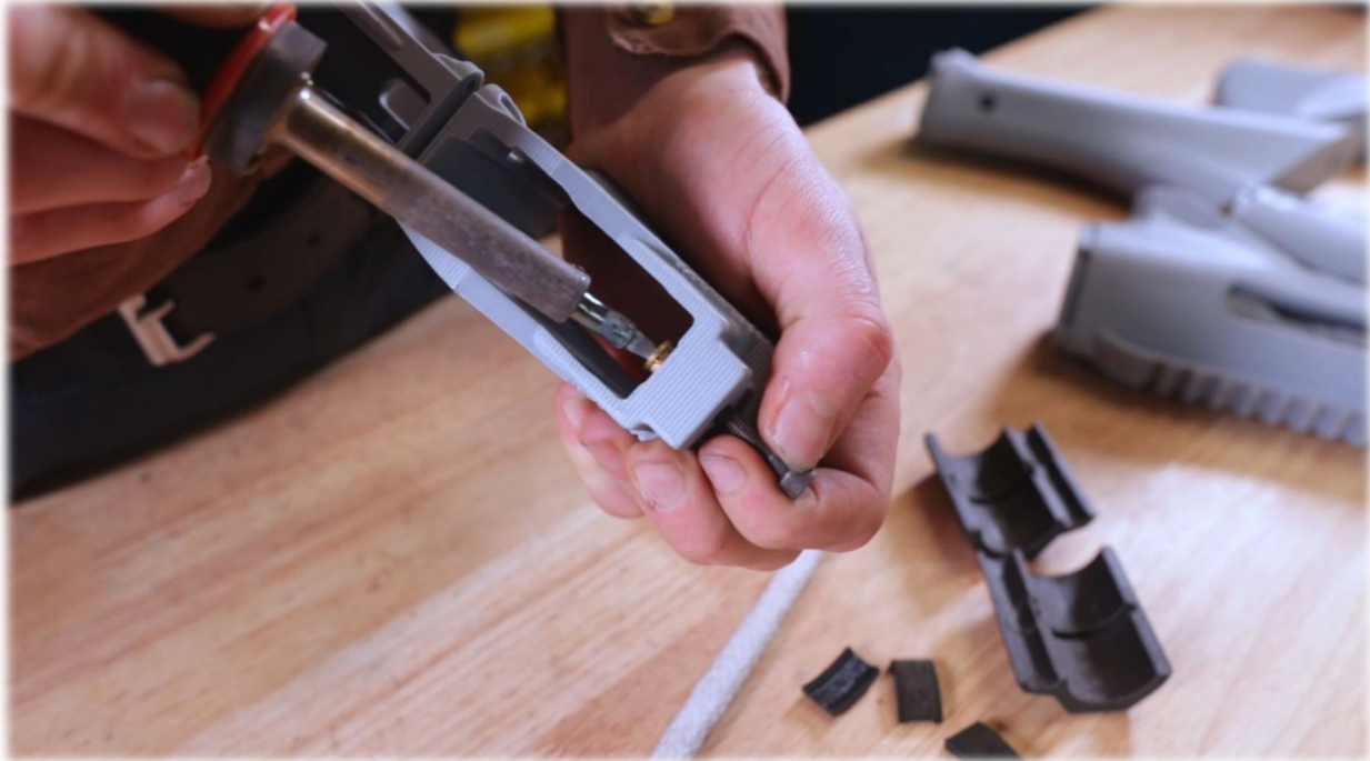
Figure 4 Installing brass insert into lower.
