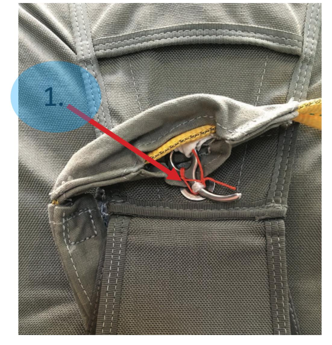
Main curved pin securing tie (must be orange and constructed of type 8/4 cotton thread) **MAIN CURVED PIN SECURING TIE - 1**
