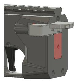
c. Install Breech onto the Receiver Front.
